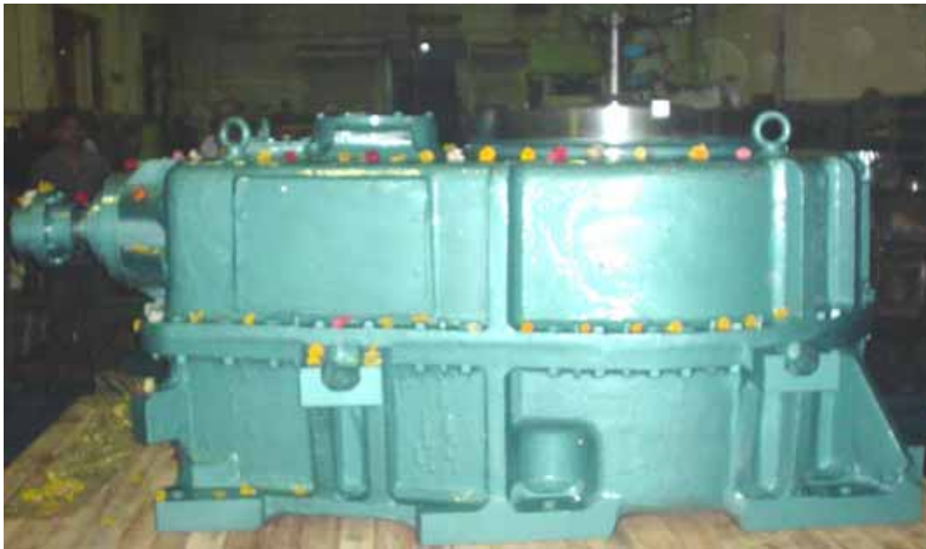
10.9 'E' Mill Gear Unit
